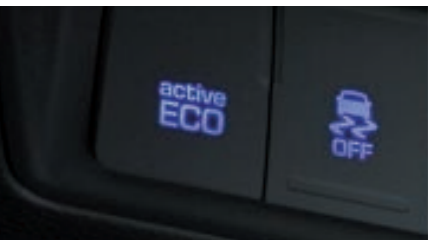
Active Eco Drive Mode Engine operating parameters can be switched to ECO mode for maximum fuel economy.
