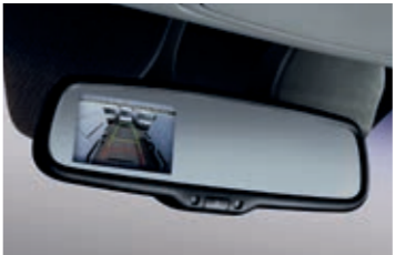
Electronic chromic mirror (ECM) with Rear camera display (RCD) The inside rear-view mirror of the wagon is an electronic chromatic type that automatically dips when dazzled by a following vehicle's headlamp main beams.
