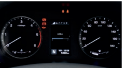
Urea Residual Gauge Tells you at a glance how much urea is left in the tank.
